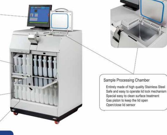
Xylene free all Intelsint tissue processors can efficently work with xylene substitutes
