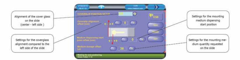
Precise setting of the coverglass on the slide and of mounting medium dispencing are provided thanks to the CVR sofisticated mounting unit.
