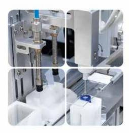
The mounting medium (500 ml bottle), is studied to be easily accessible, with rapid connections (level sensor included) which allows the operator to substitute the bottle without touching any wire.
